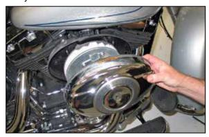
2. Remove the bolt that secures the bonnet to the filter assembly and then remove the bonnet from the vehicle.
