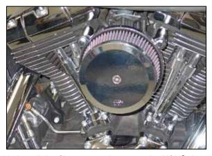
12. Install the filter cover plate onto the K&N® air filter and secure with the provided hardware. NOTE: Be sure to place one drop of thread locker to the cover plate mounting bolt.
