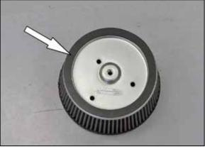
10. Install the provided gasket onto the filter top plate as shown.
