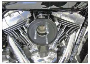
9. Install the three spacer/bolts into the K&N® filter base plate, then install the base plate gasket and one drop of thread locker onto each spacer/bolt. Install the K&N® filter base plate assembly onto the breather plate as shown.
