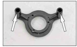
7. Install two of the provided o-rings into the K&N<sup>®</sup> crankcase breather plate as shown.
